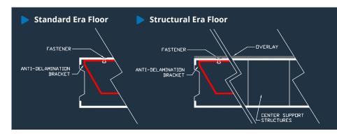
traffic. The design without plywood continues to meet NSF and DOE requirements. The Kolpak Era bracket on structural floors with the addition of 3/16" overlay provides superior strength needed for keg coolers and other heavy rolling cart loads up to 5,000 lbs. per sq. ft. uniform load.
